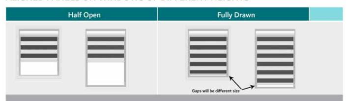
The space between the sill and the bottom bar will only have the correct clearance (approximately10mm if ordering recess) on the priority blind
