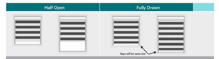
The space between the sill and the blinds will be the same (approximately 10mm if ordering recess) but the panels will not align if ordering different blind lengths
